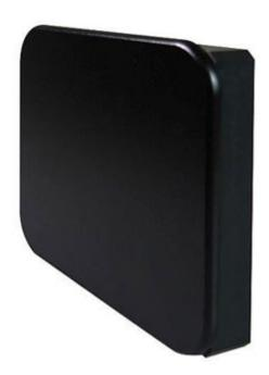
The Elatec TWN4 contactless reader is a flexible and intelligent USB unit designed for panel mounting, and that is capable of reading and writing a wide range of contactless and RFID cards and tags, operating at both 125KHz and 13.56MHz.
